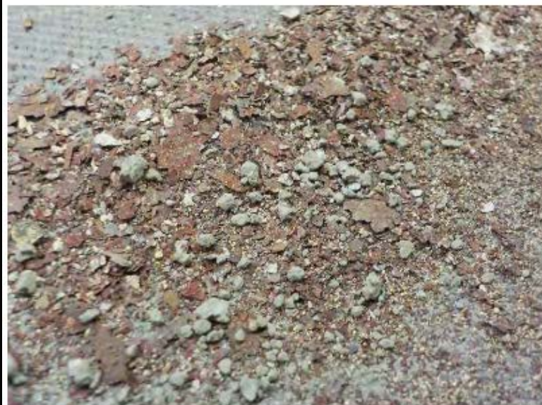
APPEARANCE OF RUST PARTICLES IN BAG BOTTOM (NON-COLLECTION SIDE)
